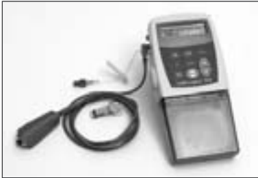
Figure 1. An electro-mechanical pump (Legacy, Deltec 6300), with patient-controlled device, for the parenteral administration of analgesics. The single-use drug reservoir is filled by the pharmacy.
